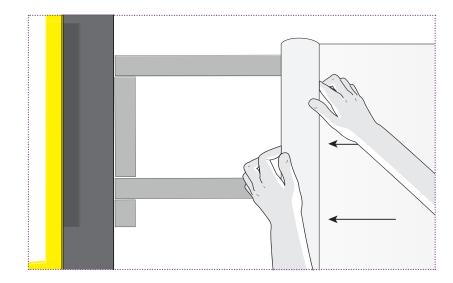
You're now ready to apply the breather membrane. Place the roll into position to cover the strips of double-sided tape and start rolling the membrane over the tape.
