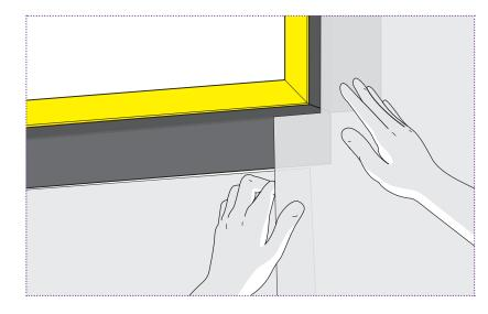
Where possible, the membrane should be continuous so any penetrations should be cut out during application, or it can be applied over the top and cut out afterwards. Horizontal laps should be 100mm and vertical laps 150mm. Vertical laps should also be staggered where possible.
